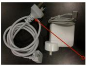
Most PC laptops have a 240V cable attached to their device power supply. Here is an example of a 240v power supply cable.
